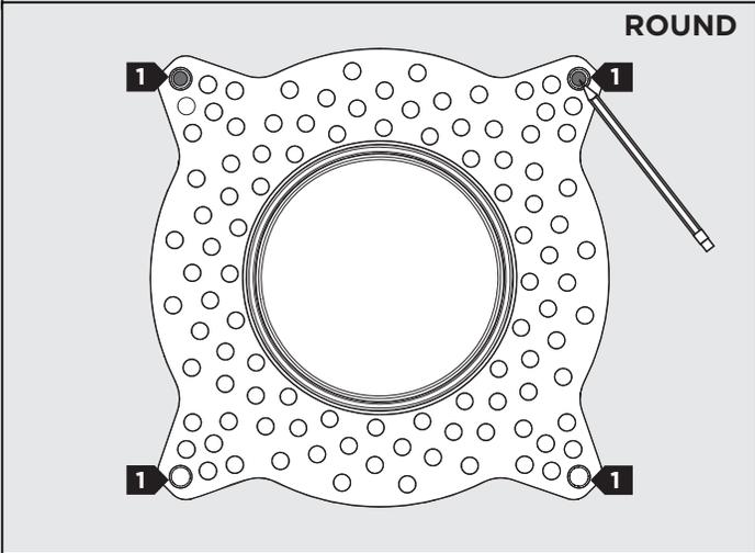
**1** Mark the location of the four mounting holes, located in the corners of the plaster ring.
