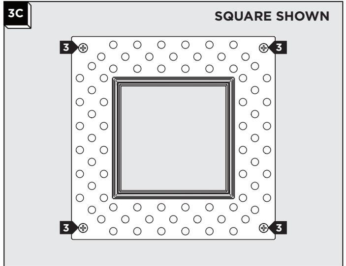
**3** Secure the plaster ring by screwing the #8 screws (1" length) screws into the anchors.
